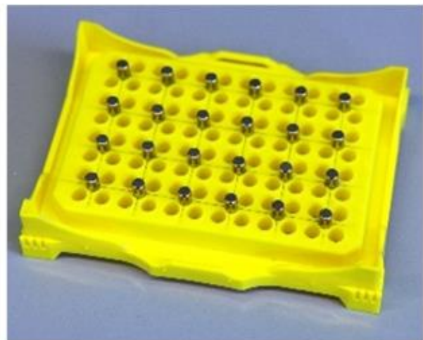
Fig 2: BOMB tubes magnetic rack can hold up to eight 1.5 ml micro-centrifuge tubes. Find the respective 3D model file on Thingiverse ( https://www.thingiverse.com/thing:3199242 ).
